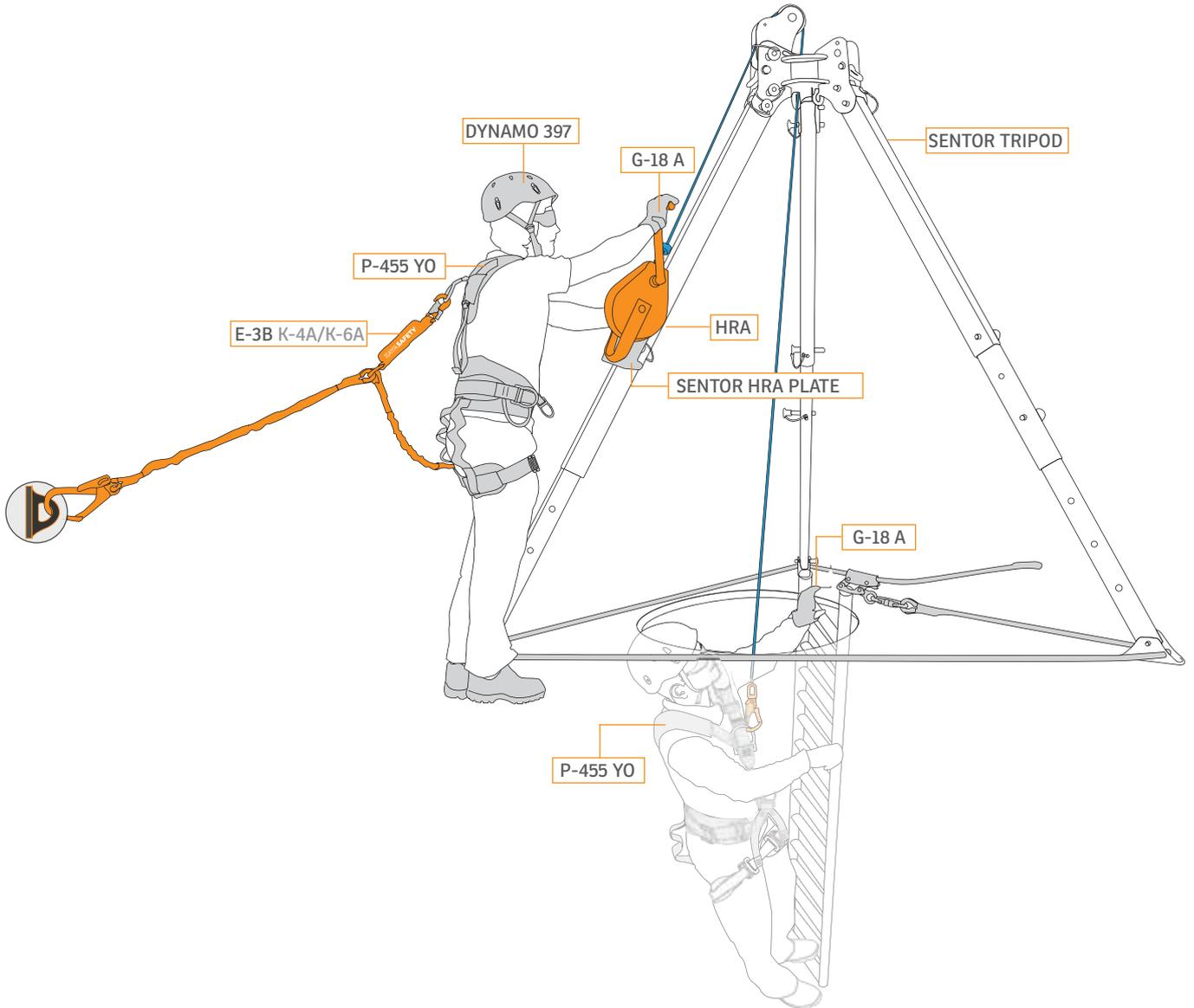
**2. WORKING IN CONFINED SPACE WITH TRIPOD AND HRA RETRACTABLE FALL ARRESTER BLOCK WITH RECOVERY MECHANISM**
