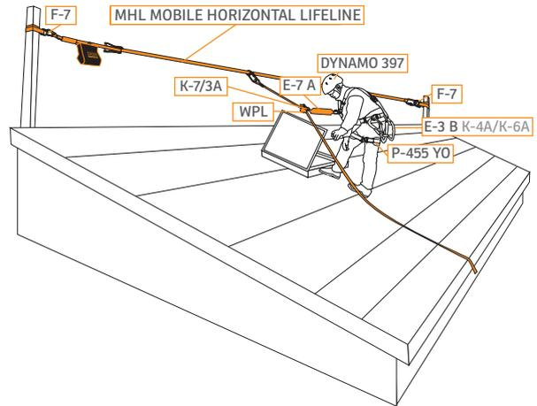
**2.1. WORKING ON MOBILE HORIZONTAL LIFELINE WITH WPL WORK RESTRAINING LANYARD**
