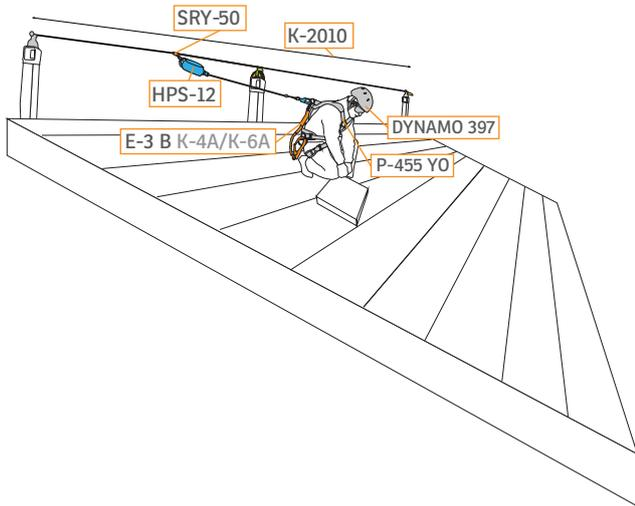
**1.1. RETRACTABLE FALL ARRESTERS LIMITS FREE-FALL DISTANCE, DECELERATION DISTANCE AND FALL ARREST FORCES WHILE ALLOWING USER FREEDOM OF MOVEMENT.**
