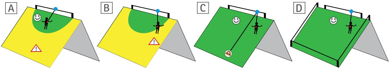
When working on the roofs with mobile horizontal lifelines, it is safe to work on the roof edges at distant points (Figure-A). When working near the edges of the roof, it must be taken a serious care against pendulum effect which will occur after a fall (Figure-B). If work is going to be performed on the sides of the roof, then l work restraining lanyard should be used in this section (Figure-C) or having safety rail on the edges would also prevent the fall (Figure-D).
