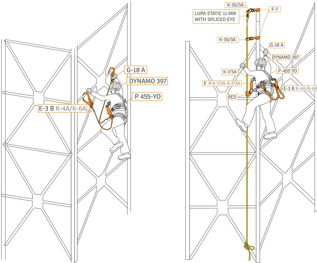
**1. ASCENDING WITH DOUBLE-LEGGED SHOCK ABSORBING LANYARD**
