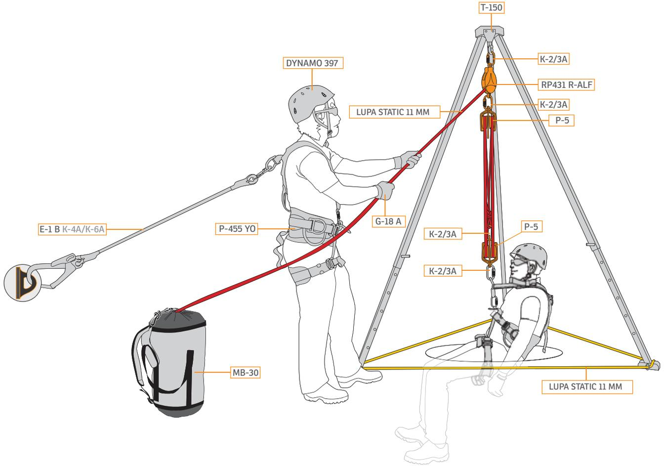
**3. WORKING IN CONFINED SPACE WITH TRIPOD AND RESCUE PULLEY**
