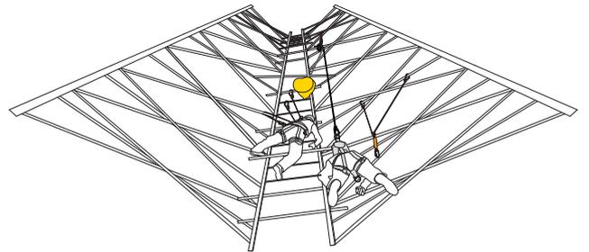
**STEP 4: TRANSFERRING SUSPENDED WORKER TO RESCUE SYSTEM**
